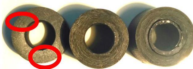
Fig. 4. Appearance of the inserts after testing (on the left – GSP, in the middle – TNC C/C, on the right – “Suvius”)
