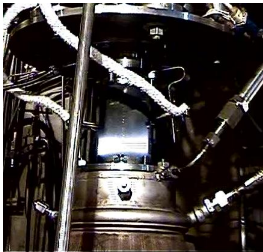
Fig. 5. Appearance of the stand for testing C-C composites with protective coating under conditions of liquid-fuel engine operation simulation
