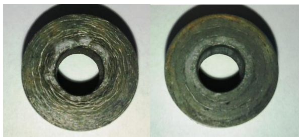
Fig. 3. Appearance of the inserts after testing on the stand (on the left – TNC C/C, on the right – “Suvius” C/C)
