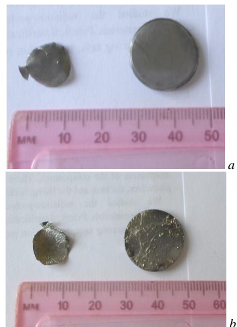
Fig. 2. Pictures of the pucks: a – before processing on the accelerator; b – after irradiation at the TEMP-A accelerator
