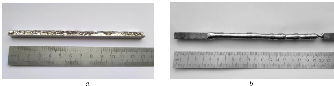
Fig. 2. The shapes of the initial iodide zirconium (a) and the metal ingot refined by the ZMEF method (b)
