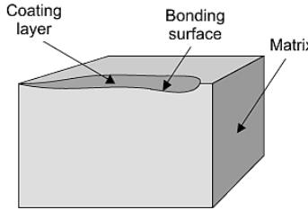
Fig. 1. Structural diagram of RM parts.
