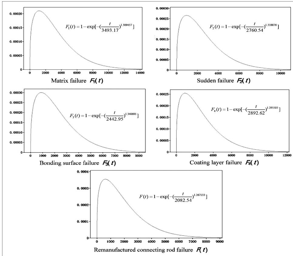
Fig. 2. Failure mechanism of polymorphic mixtures for RM connecting rod.
