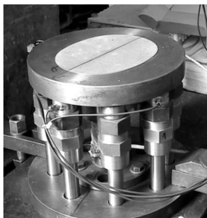
Fig. 3. Part of deep-drawing tool with TWB. Fig. 4. Tool model for deep-drawing simulations.
