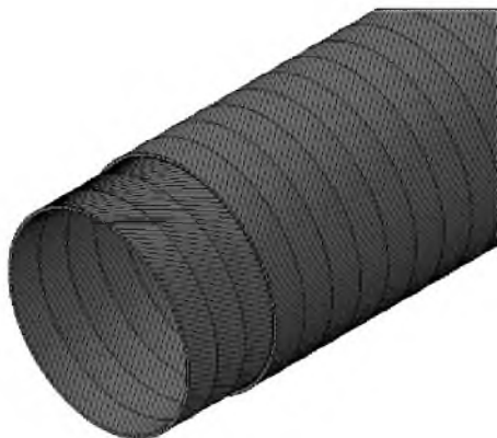
Fig. 5. Model of tension armor layers.
