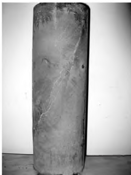
Fig. 6. Compressive failure mode of RPC in steel tubes.
