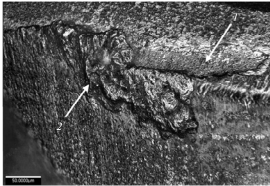
Fig. 3. Condition of cBN 8120 cutting wedge after turning at a feed rate of 0.1 mm/rev: 1 – groove; 2 – peak-up on flank face.
