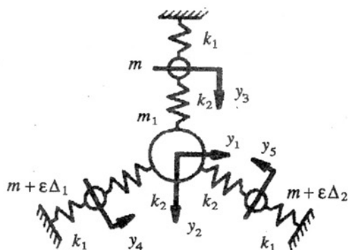
Fig. 1. Model of a mechanical system with disturbed symmetry.
