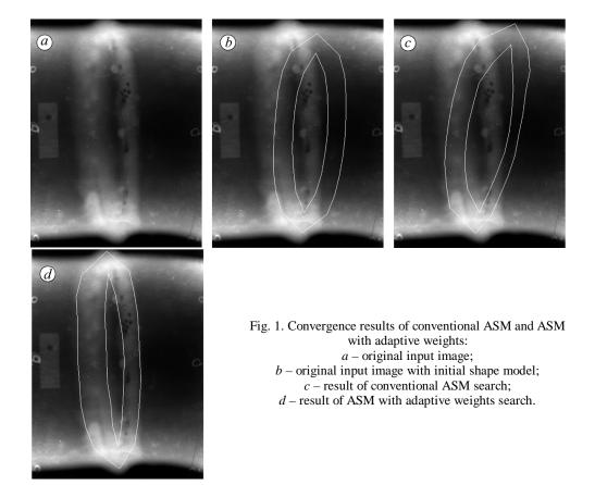
Experiments show that even though 85...95% of key points are located in proper way the model still can be lead to a wrong convergence by the small amount of key points with a big weights values. This drawback of conventional ASM can be avoided by using adaptive weights values witch are able to change during optimization stage.
