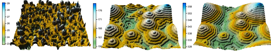
Figure 2. (Color online) Evolution of the phase field at t = 5, 30, and 60 (first second and third column, respectively). Other parameters are: \varepsilon = 4, F = 4, \mu = 10, \chi = 10, \varpi = 2, \lambda = 10, r_a = 0.01, r_b = 0.05, \vartheta = 1 .
