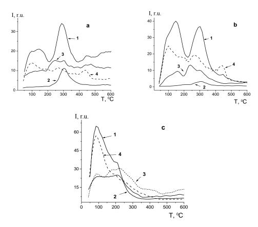
**Fig.** TD profile of CO (a), CO<sub>2</sub> (b) and H<sub>2</sub>O (c) particles for the samples:  $1 - Ni_{80}Fe_{20}$ ,  $2 - Ni_{75}Fe_{25}$ , 3 - Ni and 4 - Fe.
