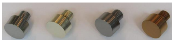
Fig. 2. Photos of Ti-6Al-4V samples without coatings and with vacuum-arc coatings
