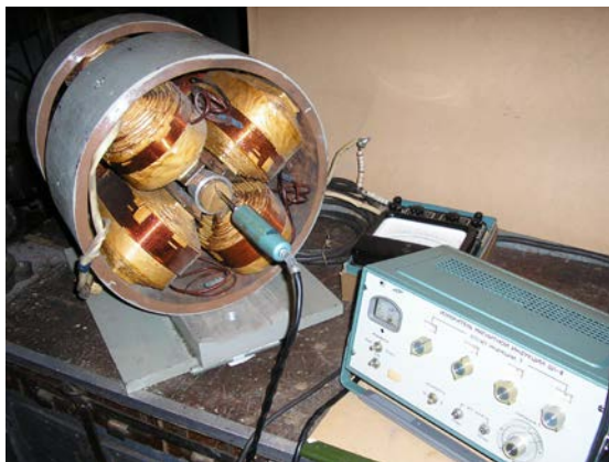
Fig. 4. A measuring complex for electromagnetic characteristics definition of quadrupole lenses
