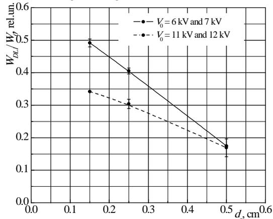
Fig. 5. Dependence of the specific energy, released in the discharge in the 1<sup>st</sup> half-period, on the high-voltage electrode diameter for the averaged values of the charging voltage
