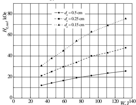
Fig. 6. Dependence of the magnetic field strength of the maximum discharge current on the initial stored energy for different high-voltage electrode diameters
