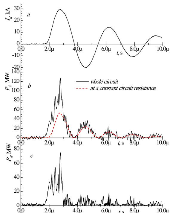
Fig. 2. Dynamics of the discharge current (a), the active power generated in the circuit (b) and inputted into the discharge (c) at a charging voltage  $V_0 = 12 \text{ kV}$  and the high-voltage electrode diameter  $d_a = 0.25 \text{ cm}$
