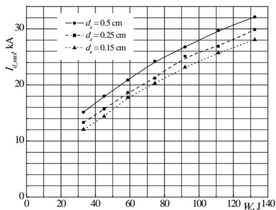
Fig. 3. Dependence of the maximum discharge current on the initial stored energy for different high-voltage electrode diameters
