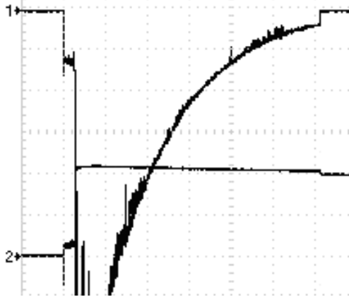
Fig. 2. The oscillograms of the collector current I (top) 2A/div; and voltage U (bottom) 10 kV/div. There is the limiting resistor of 2 k \Omega in the cathode circuit. Time scale is 1ms/div. The first 0.2 ms after the appearance of the current is in the secondary emission mode
