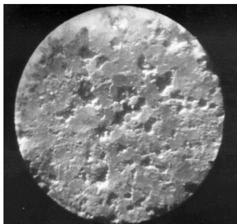
Fig. 2. Image of the porous scintillator (optical microscope MBS-9, \times 6 ).
