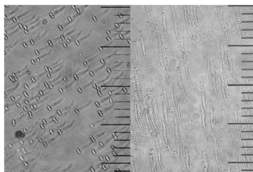
Fig. 2. Microphotos of the SiO 2 matrix in two planes in transmitted light (1 graduation line is 0.01 mm).
