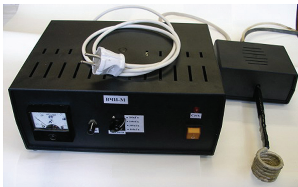
Fig. 1. Experimental setup consisting of a high frequency generator (a) and coil (b)
