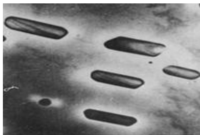
Fig. 4. Morphology of the boride phase \text{Ni}_3\text{B} , \times 45000
