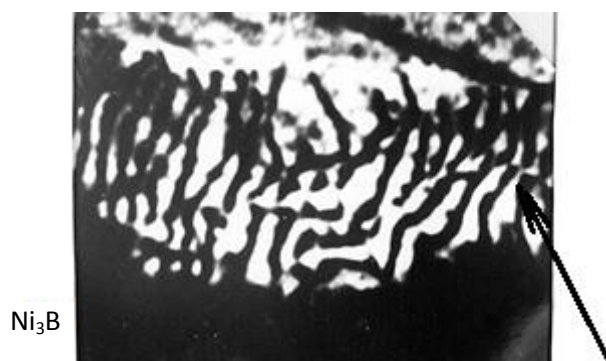
Fig. 6. Dislocation disparities in nickel-boron alloys (shown by an arrow), \times 50000
