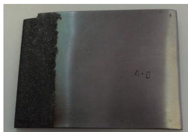
Fig. 3. A sample of a blade strengthened with 15X11MΦ-III steel by the method of electrospark alloying
