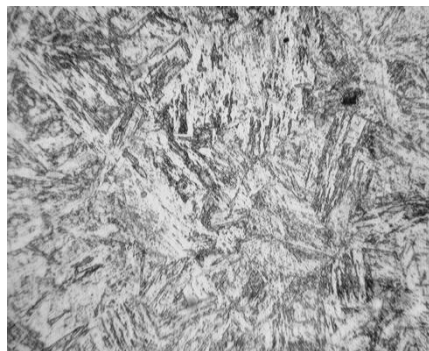
Fig. 4. Microstructure of the blade sample parent metal, x100
