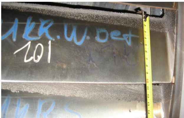
Fig. 16. Blades hardened with T15K6 alloy by electrospark alloying method
