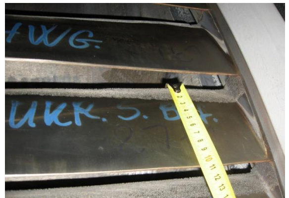
Fig. 17. Blades hardened with 15X11MΦ-III steel by electrospark alloying method
