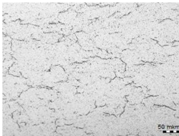
б – 140 ppm, P_{293}=5,0 МПа, \sigma_{\theta} при 450^{\circ}\text{C}=76,7 МПа, N_{\text{циклов}}=3, F_{\text{H}}\approx 0,1
