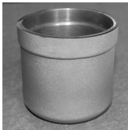
Fig. 5. A crucible made of fluoride-originated tungsten.
