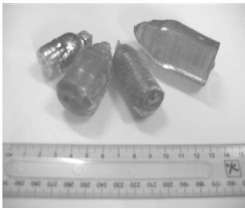
Fig. 5. \text{ZnMoO}_4 single crystals.
