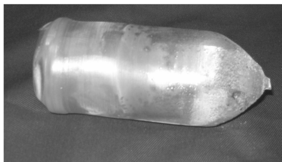
Fig. 1. CdWO 4 single crystal (3 kg).
