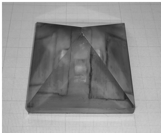
Fig. 1. As grown KDP single crystal doped with Xylenol orange dye.
