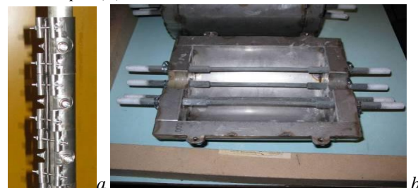
Fig. 7. Cup-type (0.4 kW, 100 mm working length) heater (a) and radiation-type (up to 10 kW, 310 mm internal working length) heaters with silit heating elements (b)
