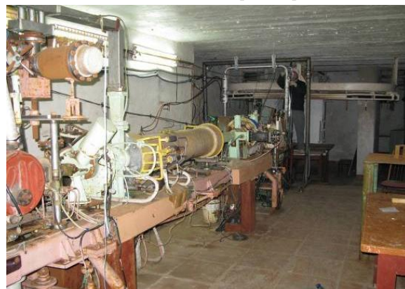
Fig. 1. Placement of the SCWCL in the bunker room of the LPE-10 electron linac
