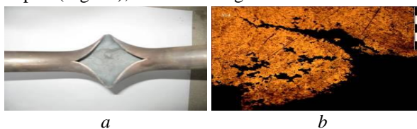
Fig. 10. Top view at the point of rupture of the SCWCL prototype pipe (a) and the \times 200 magnification cross section electron microscopy along the specimen break
