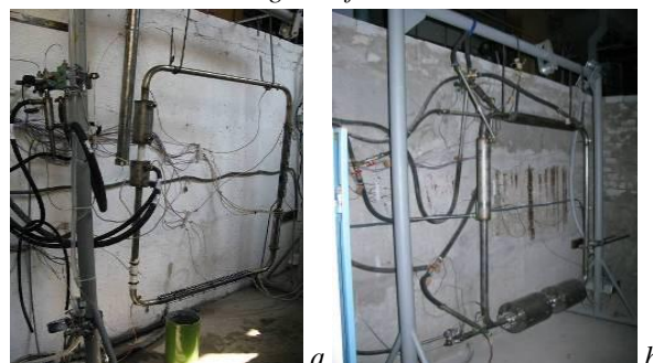
Fig. 6. The SCWCLs Loop-1a with cup-type heaters (a) and Loop-1 (b) with radiative heaters on the test stand
