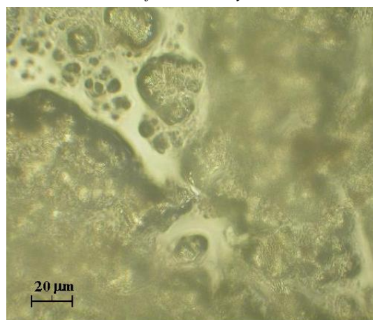
Fig. 5. A microphotograph of the immersion preparation of the irradiated sample KMgPO 4 ·6H 2 O (D=1.35·10 5 Gy) in transmitted light. Without analyzer
