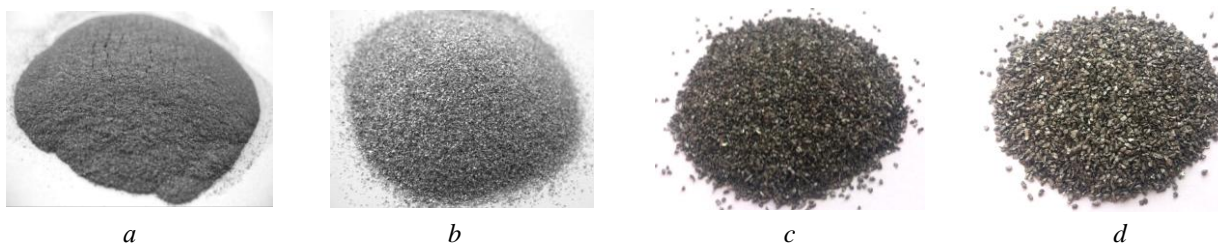
Fig. 6. Appearances of aluminium alloy powder fractions: a – 50...112; b – 112...315; c – 500...700; d – 800...1000 μm
