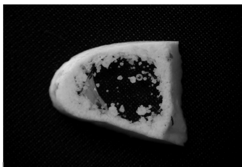
Fig. 3. Crystallization of the glass (0.8·SrB 4 O 7 -0.2·PbB 4 O 7 ) an initial stage in isothermal conditions.
