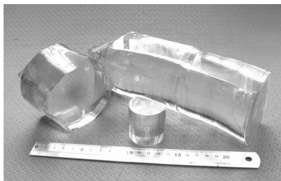
Fig. 2. Large-size \text{ZnWO}_4 crystal.
