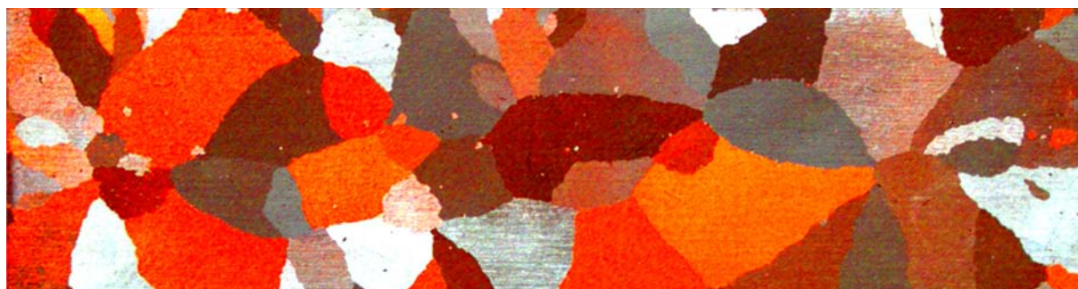
Fig. 1. Color orientation map of an aluminum polycrystal surface ( \times 2 ), the whole sample.
