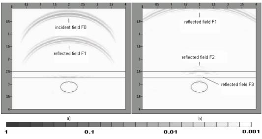
**Fig. 3.** Distribution of the field component  $E_x$  in space at the time a) t = 150 time-steps; b) t = 250 time-steps
