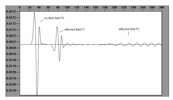
**Fig. 5.** Distribution of the field component  $E_x$  at the point (100, 110) during 300 time-steps
