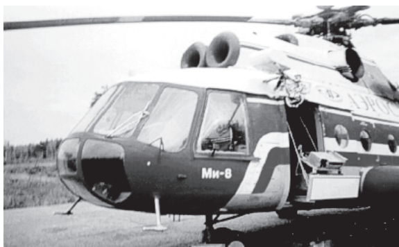
Fig. 14. The dual frequency radar system installed on a helicopter
