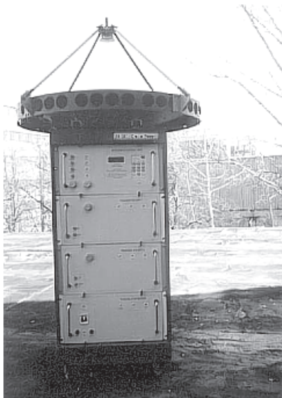
Fig. 6. Transmitter-receiver rack together with the radar antenna
