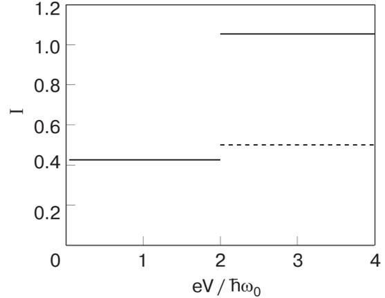
Fig. 3. The current as plotted as a function of the bias voltage (solid line). The current makes a jump as the non-elastic channel is opened at  $V = 2\hbar\omega_0/e$ . We have also plotted (dashed line) the current as a function of voltage for the high dissipation limit where the harmonic oscillator goes to the ground state between tunneling events.
