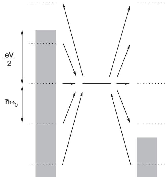
Fig. 2. Illustration of the second order case where elastic tunneling and inelastic tunneling exchanging two or less vibrational quanta are included. The level of the dot is equal to the chemical potential and the bias voltage is set so that  $2\hbar\omega_0/e < V < 4\hbar\omega_0/e$ .
