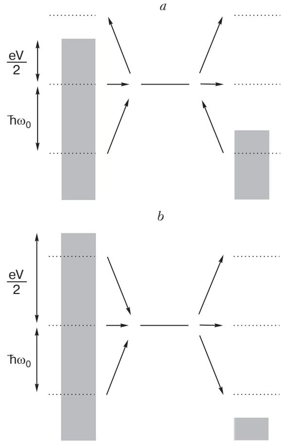
Fig. 1. Model system consisting of a one level quantum dot placed between two leads. The level of the dot equals the chemical potential of the leads and a bias voltage of  $V$  is applied between the leads. The center of mass movement of the dot is in a harmonic oscillator potential with the vibrational quanta  $\hbar\omega_0$ . The applied bias voltage is such that  $eV/2 < \hbar\omega_0$  (a). Same as (a) but with the applied bias voltage larger than  $2\hbar\omega_0/e$  (b).
