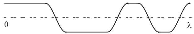
Fig. 2. The wave is composed of alternating two flat segments of different lengths and four kinks of width l/2 each.
