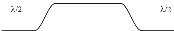
Fig. 1. The wave is formed by alternating one flat segment of length (\lambda - l)/2 and kink of width l/2 .
