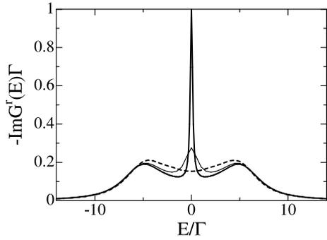
**Figure 7.** The spectral function with the second-order self-energy at  $U/\Gamma = 10.0$  for the symmetric Anderson model at equilibrium (solid line),  $eV/\Gamma = 1.0$  (thin solid line) and  $eV/\Gamma = 2.0$  (dashed line).
