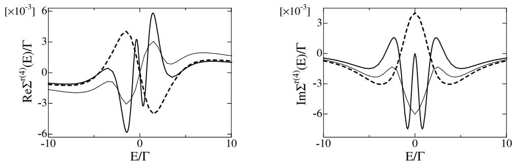
**Figure 6.** The fourth-order self-energy for the symmetric Anderson model at  $U/\Gamma = 1.0$  and zero temperature. (a) The real part and (b) the imaginary part at equilibrium (solid line),  $eV/\Gamma = 1.0$  (thin solid line), and  $eV/\Gamma = 2.0$  (dashed line). The fourth-order contribution for equilibrium has the same but narrow curves at low energy with those of the second-order contribution.
