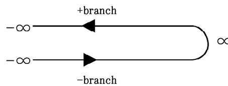
**Figure 1.** The time-contour which starts and ends at  $t = -\infty$ .
