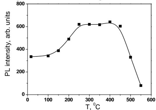
**Fig. 3.** Influence of isochronous annealing in Ar ambient on the PL intensity of na-Si/SiO<sub>x</sub> porous column-like nanocomposite films.
