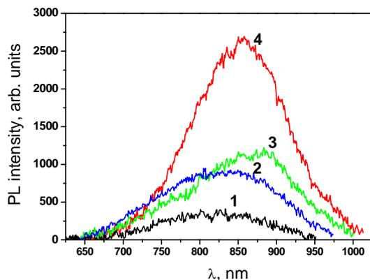
**Fig. 1.** Influence of type of gas ambient on PL spectra (1 – initial sample without low-temperature annealing, 2 – after annealing in H<sub>2</sub> ambient, 3 – in Ar and 4 – in N<sub>2</sub>).
