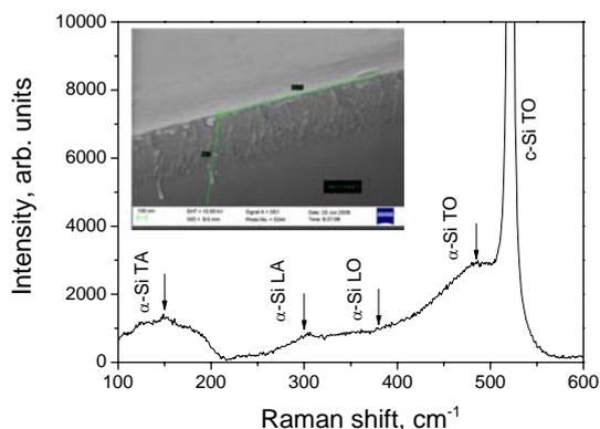
**Fig. 2.** Raman spectra and SEM micrographs (insert) of na-Si/SiO<sub>x</sub> porous column-like nanocomposite films
