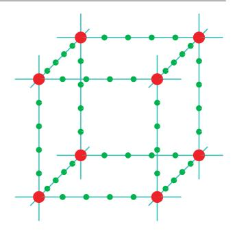
*Fig. 1.* Elementary cell of the decorated lattice (q = 5). Large circles represent central sites, small ones, the internal sites of the segments.
