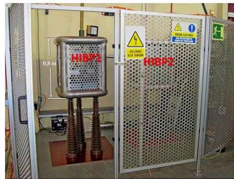
Fig. 7. Exterior view of the injector control and power supply systems for the HIBP1 and HIBP2 diagnostics on the TJ-II stellarator
