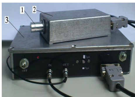
Fig. 3. Experimental setup used in Gd measurements: 1 – detection module; 2 – preamplifier (2×2×6 cm), and 3 – the power supply
