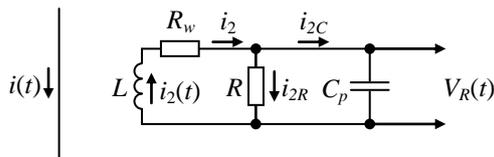
Fig. 2. The equivalent scheme of the integrating current transformer:  $i_1(t)$  – the measured and  $i_2(t)$  – the inducible currents;  $V_R(t)$  – the observed signal;  $R_w$  – the coil wire and  $R$  – the measuring resistance;  $L$  – the coil inductance;  $C_p$  – the parasitic capacity
