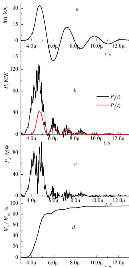
Fig. 4. Dynamics of the discharge current (a), the total active power in the circuit (b), the additional active power released in the discharge (c) and the absorbed energy (d)
