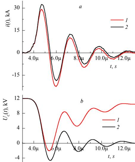
Fig. 3. The dynamics of the discharge current (a) and the dynamics of the capacitor bank discharge (b) for the observed (1) and restored (2) signal
