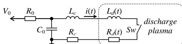
Fig. 1. The equivalent scheme of the discharge circuit
