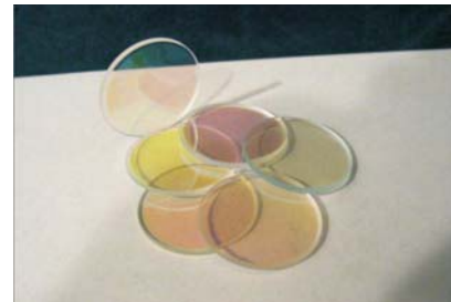
Fig. 3. Experimental specimens of the optical elements for the IR narrow-band filter with the multilayered coatings on the base of MgF_2-LuF_3 and ZnS-GdS composites (CDO "Arsenal")
