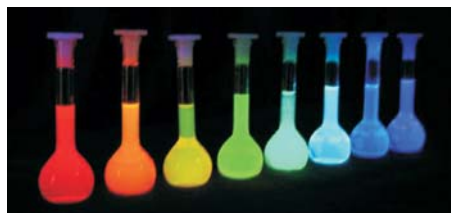
Fig. 1. Seta and Square dyes fluoresce in a wide spectral region from the ultra-violet (UV) to the near-infrared (NIR)
