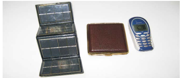
Fig. 2. Folding solar array for mobile phones SBMT-S-8.0-0.23 (experimental sample) and its case
