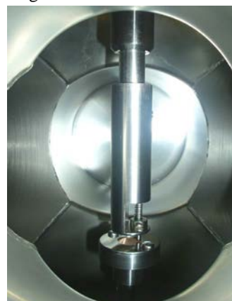
Fig. 4. The cathode-holder with the sample and anode in the vacuum chamber
