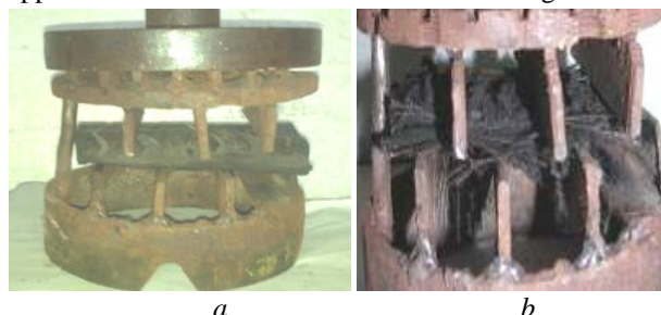
Fig. 3. Tire sample in the module for the application of mechanical load (a – before the disintegration process; b – after the disintegration process)
