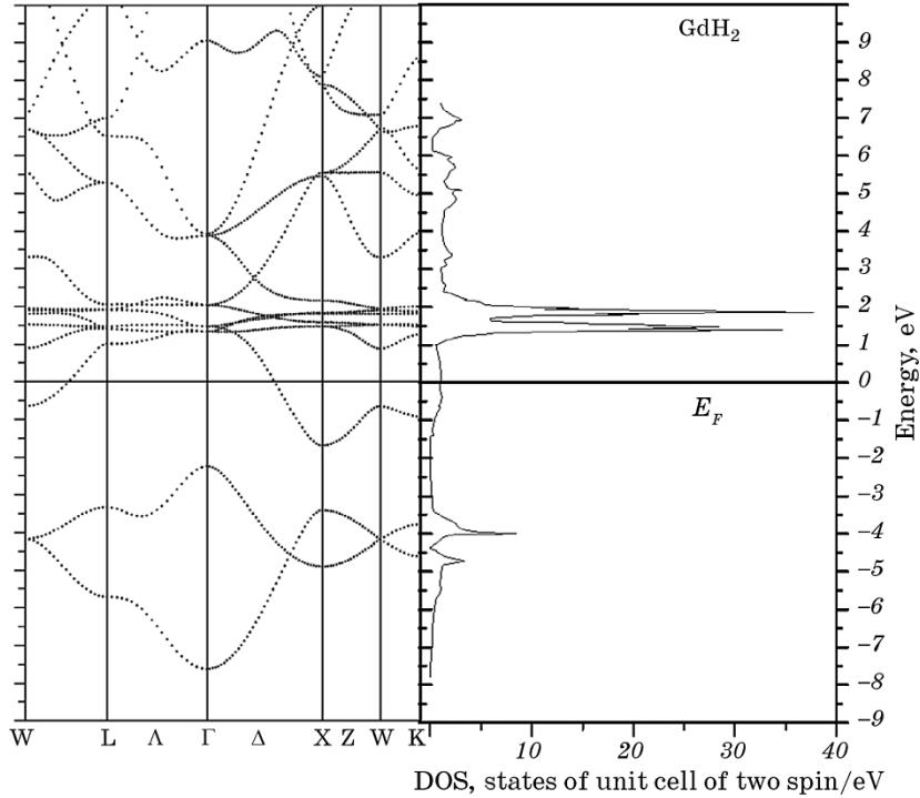
**Fig. 5.** Density of states (right panel) and electronic band structure along high-symmetry directions (left panel) of  $\text{GdH}_2$ , the Fermi energy being at 0 eV.
