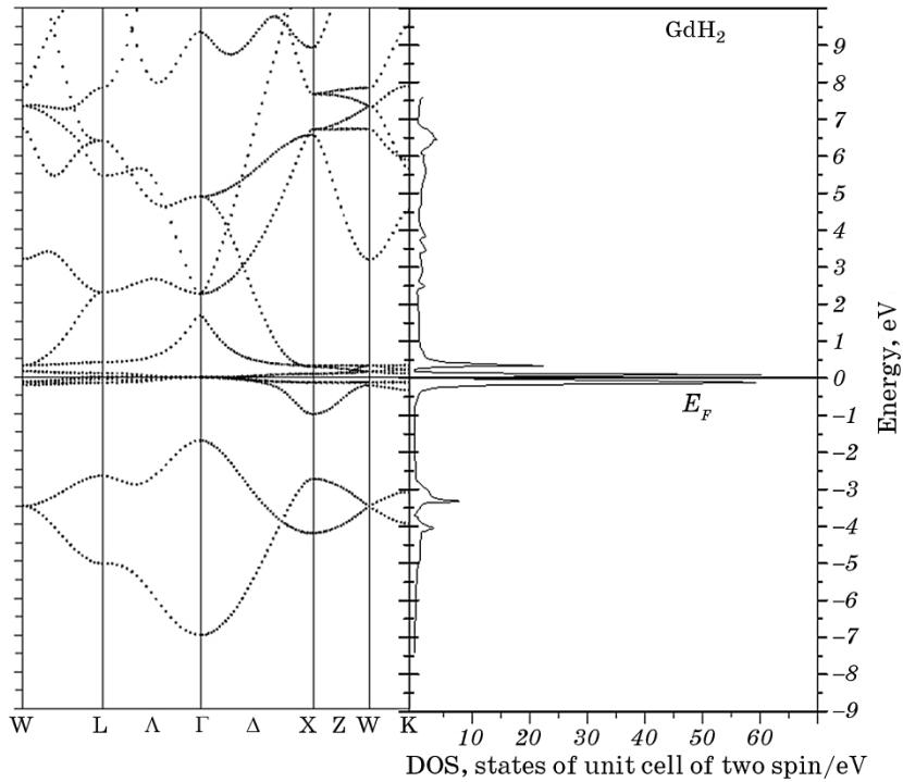
**Fig. 4.** Density of states (right panel) and electronic band structure along high-symmetry directions (left panel) of  $\text{GdH}_2$ , the Fermi energy being at 0 eV.
