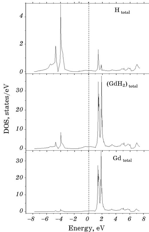
**Fig. 8.** The calculated total and partial density of states for  $\text{GdH}_2$ .
