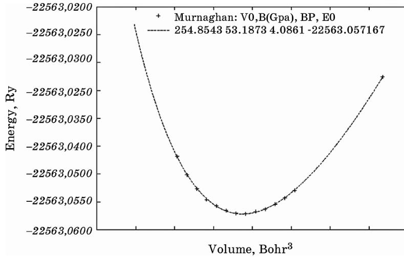
**Fig. 3.** Total energy of  $\text{GdH}_2$  as a function of volume.
