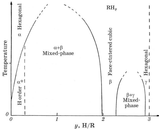
**Fig. 1.** Typical phase diagram of R–H systems.
