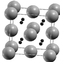
**Fig. 2.** The compound crystallises in the  $\text{CaF}_2$  fluorite type structure: the large spheres represent rare earth atoms ( $\times 4$ ) and small spheres hydrogen atoms occupying tetrahedral sites ( $\times 8$ ) (figure plotted with XCrySDen [3]).
