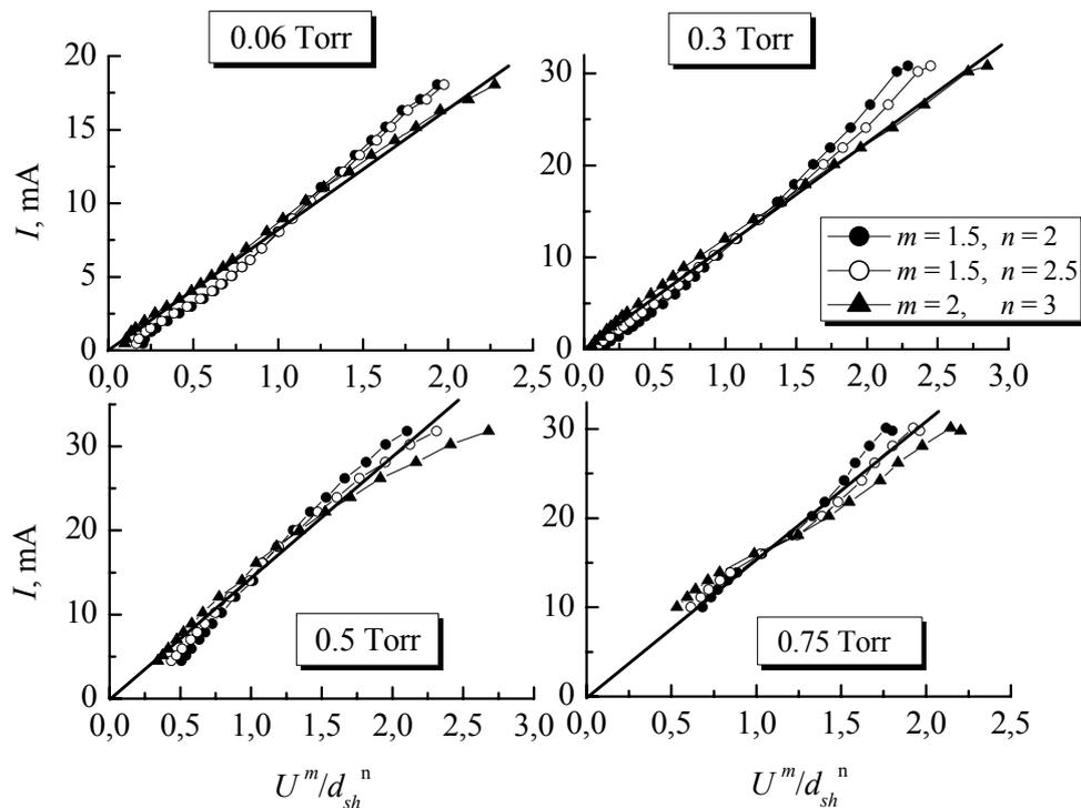
Fig. 3. Discharge current against  $U^m/d_{sh}^n$  ratio ( $m = 1.5, n = 2$ ;  $m = 1.5, n = 2.5$ ;  $m = 2, n = 3$ ) for different  $N_2O$  pressure values. Inter-electrode difference is 20 mm
