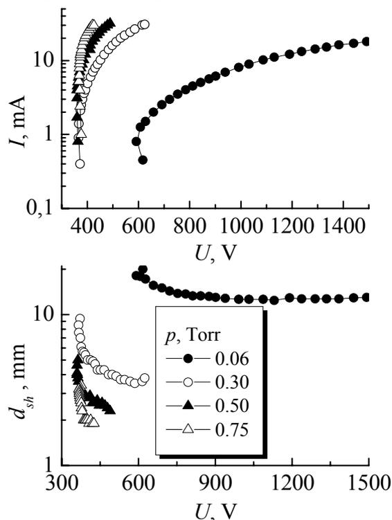
Fig. 2. Discharge current and cathode sheath thickness against voltage for different  $N_2O$  pressure values and the inter-electrode distance of 20 mm
