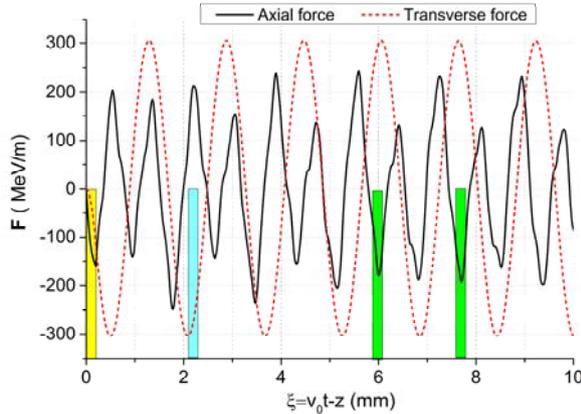
Fig. 1. Axial profile of the axial force (black line) and axial profile of transverse force (red line) at the distance  $r=0.45 \text{ mm}$  from waveguide axis. Drive bunch (yellow rectangle) moves from right to left. Cyan rectangle shows possible location of electron witness bunch and green rectangles show possible location of positron witness bunch. Plasma density  $n_p = 3n_b$
