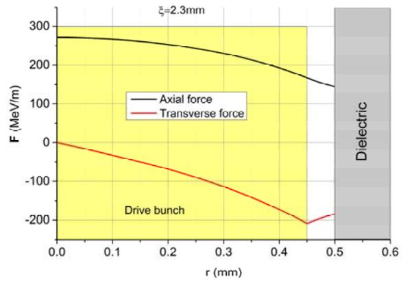
Fig. 2. Transverse profile of the longitudinal force (black line) and transverse one (red line), acting on a witness electron, located at a distance of  $2.3 \text{ mm}$  ( $\xi \equiv v_0\tau = v_0t - z$ ) from the head of the drive bunch
