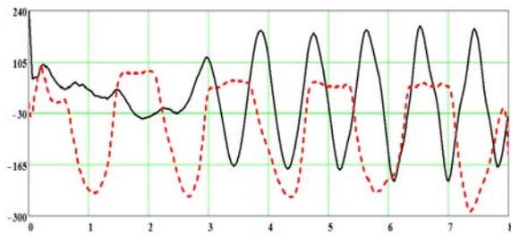
Fig. 3. Axial profile of the axial force (black line) and axial profile of transverse force (red line) at the distance  $r=0.45$  mm from waveguide axis at time  $t=26.688$  psec. Drive bunch moves from left to right, its head is located at  $z=8$  mm. Distance ( $x$ -axis) is measured in mm, forces ( $y$ -axis) are in MeV/m
