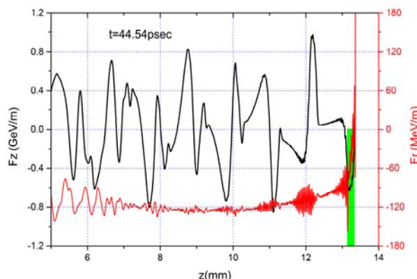
Fig. 6. Axial profile of the axial force (black line) and axial profile of transverse force (red line) in the case of blowout excitation regime of plasma-dielectric waveguide:  $n_b/n_p = 30$ . Forces are recorded at the distance  $r=0.1$  mm from waveguide axis at time  $t=44.54$  psec. Drive bunch moves from left to right, its location is shown green rectangle
