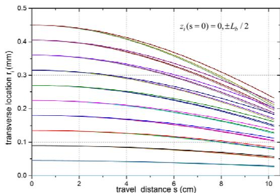
Fig. 7. Radii of witness bunch electrons during the acceleration by wakefield of drive bunch. Initially (at  $s=0$ ) center of witness bunch is located at the distance of 2.2 cm behind of drive bunch head
