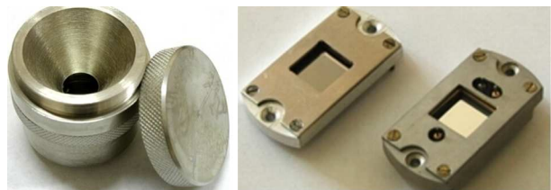
Fig.3. General view of detector head and silicon PIN-detectors
